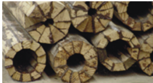
Figure 3. Laminated utility poles constructed from decommissioned preservative-treated wood.
