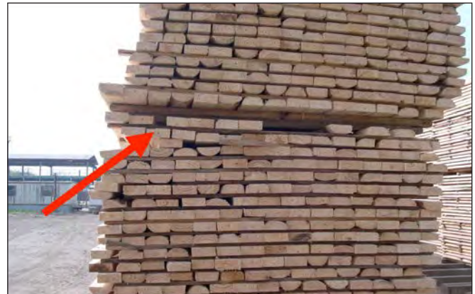
Figure 3. Notice how this stack of southern pine lumber is leaning due to the bowing of several boards. The central core, or pith, is readily identifiable in many of the boards, indicating the presence of juvenile wood.
