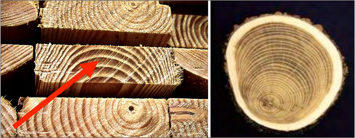
Figure 2. Compression wood as viewed in pine lumber (left) and tension wood inside a hardwood tree (right).
