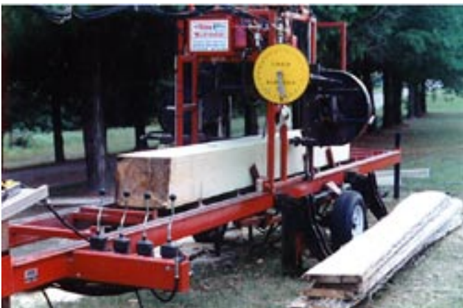
Portable sawmills are often used to saw trees into lumber from small woodlots.
